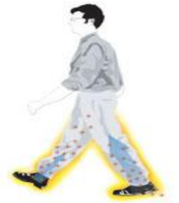
Friction between two materials, such as a shoe sole and flooring, can generate a walking charge.
