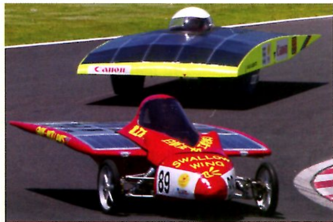
Figure E These cars are powered by photons which strike the solar cells on their surface.
