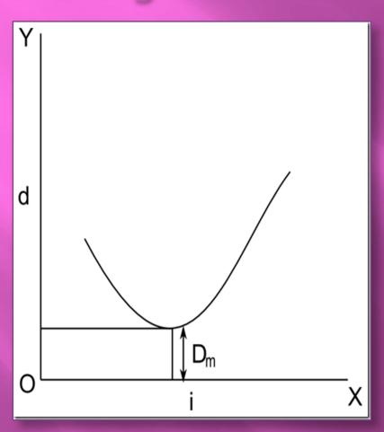
As the angle of incidence increases, the angle of deviation goes on decreasing till for a certain angle of incidence it attains the minimum value which is known as angle of minimum deviation. When the angle of incidence is increased further, the angle of deviation now starts increasing.
