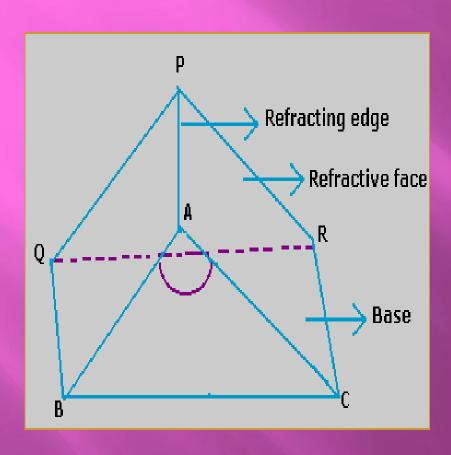
A prism is a transparent refracting medium Bounded by two plane surfaces making an angle with each other.
