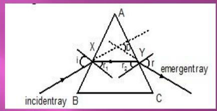
A light ray striking at one face of a triangular glass prism gets refracted twice and emerges out from the other face as shown above. The angle between the emergent and the incident rays is called the angle of deviation (D). The angle between the two refracting faces involved is called the refracting angle (A) of the prism.
