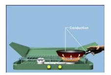
When a solid is heated, the molecules start vibrating about their mean position. The vibrating molecules collide with the neighbouring molecules, as a result the vibration of the neighbouring molecules increases.
