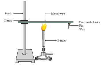
The above activity shows that metals are good conductors of heat. The best conductors of heat are silver and copper. Lead and mercury are comparatively poor conductors of heat.
