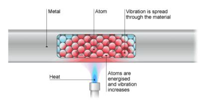
When we hold a metal rod near the candle flame as shown in the figure, the end of the rod closer to the flame becomes hot first and the heat is transferred to the cooler end of the rod. Thus heat is transferred from one end of the rod to the other end.
