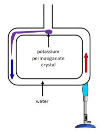
You can also use the special piece of apparatus shown in the diagram. It is a "square "glass tube filled with water. Drop a crystal of potassium permanganate into the top and then heat one of the bottom corners gently. You will see the colour begin to move round the tube going down the limb opposite the heating and then rising up the other side above the Bunsen due to convection currents in the water.
